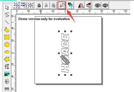
4. Press "Hatch" button to fill in the text.
