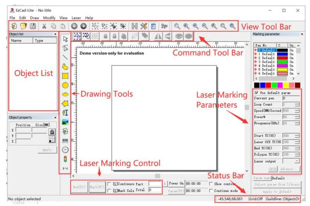
Hoace Intelligent UV Laser marking machine is controlled by the included EZCad2 Lite software, which must be installed on a compatible computer to direct the laser. See its separate instruction for full details on its components and use. Some features which are particularly important to note include the following parameters and controls:
