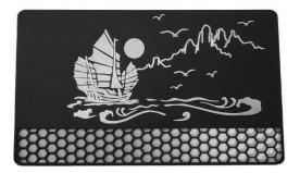
**Step 10.** Replace the test material with the actual material. Use the foot pad or press Mark or hit F2 in EZCad2 Lite to engrave your pattern. Again, do not stare at the laser in operation even with protective eyewear. Watch for possible issues like sparks or fires, however, and be prepared to quickly extinguish a fire if necessary.
