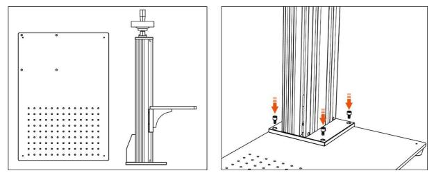
**Step 2.**Adjust the nut at the bottom of the light path to an appropriate position. Install the light path onto the lifting column using the provided screws. Tighten the four screws with the Allen key.
