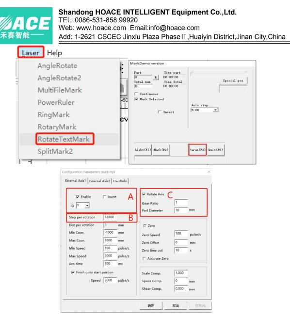
A. Enable extended axis, reverse mode, enable Y axis (enable X or Y axis according to the direction in which the rotation axis is placed).
