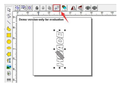
4. Press "Hatch" button to fill in the text.
