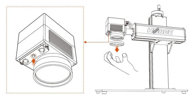
Step 6. Turn the focus wheel to adjust the two red dots to coincide to achieve focus.
