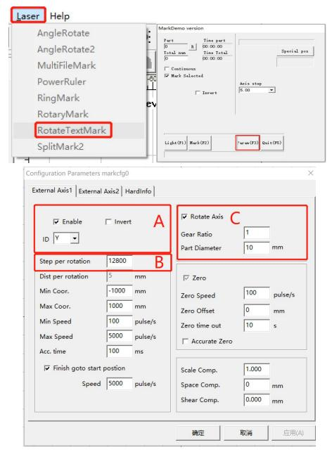
A. Enable extended axis, reverse mode, enable Y axis (enable X or Y axis according to the direction in which the rotation axis is placed).
