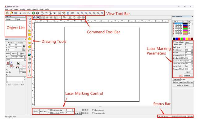
Hoace Intelligent MOPA Fiber Laser Mrking Machine is controlled by the included EZCad2 software, which must be installed on a compatible computer to direct the laser. See its separate instruction for full details on its components and use. Some features which are particularly important to note include the following parameters and controls:
