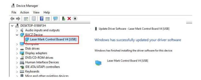
Now you see the driver "Laser Mark Control Board V4 [USB]" was installed successfully.
