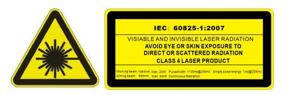
When the red radiation produces refraction to eyes, it will focus on the retina, eyes will be hurt easily. In a word, you should always wear protective glasses during the machine operation or maintenance.
