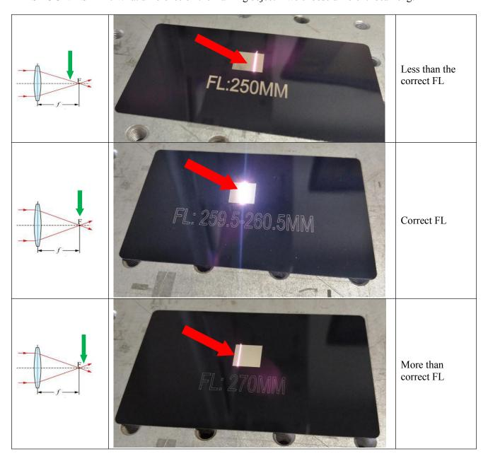
After checking the above pictures, we will see: when we use the wrong FL for marking object, then we can not get the strongest laser power.
