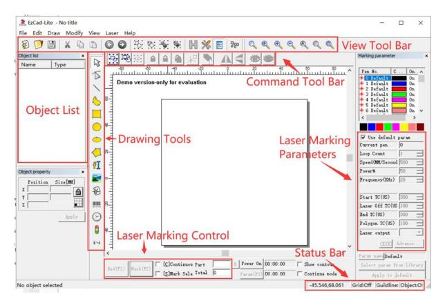
Hoace Intelligent Co2 Laser marking machine is controlled by the included EZCad2 Lite software, which must be installed on a compatible computer to direct the laser. See its separate instruction for full details on its components and use. Some features which are particularly important to note include the following parameters and controls:
