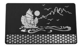
**Step 10.** Replace the test material with the actual material. Use the foot pad or press Mark or hit F2 in EZCad2 Lite to engrave your pattern. Again, do not stare at the laser in operation even with protective eyewear. Watch for possible issues like sparks or fire, however, and be prepared to quickly extinguish a fire if necessary.
