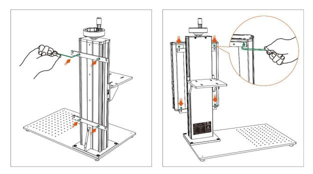
**Step 3.** Adjust the nut at the bottom of the light path to an appropriate position. Install the light path onto the lifting column using the provided screws. Tighten the four screws with the Allen key.
